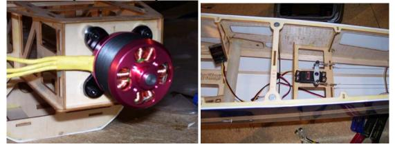
The cowl was attached with four wood screws, I preferred to substitute #2 allen-head style button heads per my preference while lining up the cowl with the Hyperion Spinner that I got from 3D Hobbyshop. I attached the wings with the supplied nylon wing bolts, routed the wires, and mounted the Rx and battery Velcro, a quick program in the radio and Bingo! We are flight ready!
