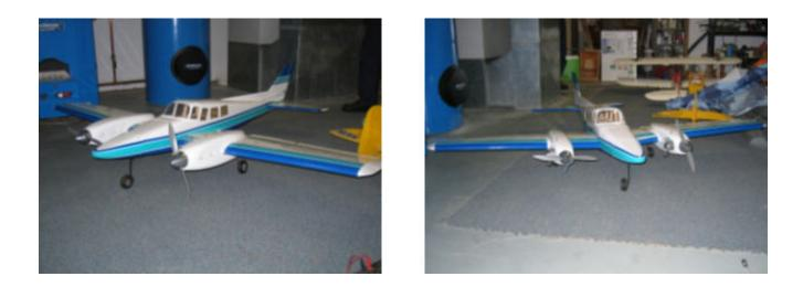
Fred Meyer brought in a Goldberg Ultimate built from a kit in 1998 and covered the winter of 2006. Power is by a Super Tiger .90 turning a 14 x 6 prop. The Elevator and Rudder are Push-Pull and use Hitec 5625 Digital Servos. Three Futaba S148's converted to 2 BB are used for the ailerons. & throttle. A six-volt receiver pack is used with a Futaba FM receiver.
